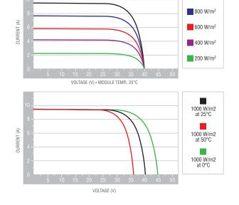
\*STC: (Standard Test Condition) Irradiance 1000W/m²; Module Temperature 25°C; Air Mass 1.5
